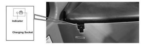
Charging socket is near the seat. Plug in the charger, then connect the charger with power.
