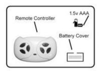
Remove the cover screw and battery cover. Insert 2 x AAA 1.5V batteries, observing the polarity. Replace the cover and secure the screw.
