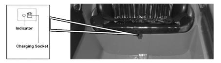
Charging socket is near the seat. Plug in the charger, then connect the charger with power.
