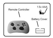
Remove the cover screw and battery cover. Insert 2 x AAA 1.5V batteries, observing the polarity. Replace the cover and secure the screw.
