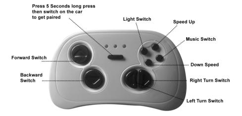
\* Remote control has range approx 15~20m. If remote does not perform properly within this coverage please check battery.
