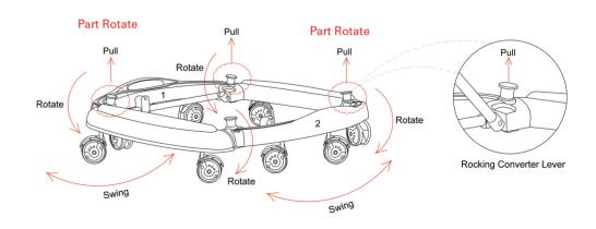
Pull Both the Rocking Converter lever of each side at the same time. White Keep Pulling the lever; rotate part downward.
